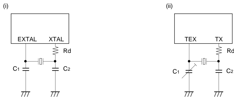
Fig. 11. SPC700 Series recommended oscillation circuit
